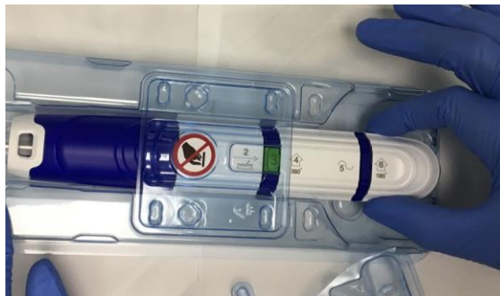
Figure 4. Pull device handle back to firm stop.
